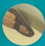
**2a.** Remove Blending Disc from backup pad to sand hard-to-reach areas and edges.
