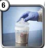
Take a lid (with built-in filter) from wall dispenser and snap into the 3M<sup>™</sup> PPS<sup>™</sup> cup/liner.
