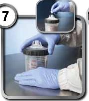
Position locking collar onto the 3M<sup>TM</sup> PPS<sup>TM</sup> cup/liner and turn until tight. Insert sealing plug prior to shaking.
