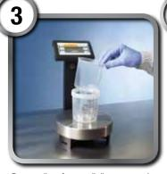
Remove liner from wall dispenser and place into 3M<sup>TM</sup> PPS<sup>TM</sup> mixing cup. Weigh the paint according to paint manufacturer's guidelines.
