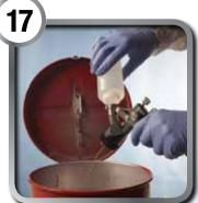
A squeeze bottle (Part No. 37720) containing solvent or water enables fast gun cleaning once the 3M<sup>TM</sup> PPS<sup>TM</sup> cup is removed. More efficient painters make shops more productive.
