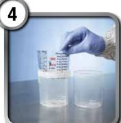
If not using a scale to measure, insert 3M<sup>TM</sup> PPS<sup>TM</sup> Mix Ratio Film into cup before inserting liner in order to measure the paint according to paint manufacturer's guidelines.
