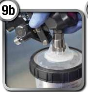
Make sure that the lid fingers are fully engaged above adapter edge.
