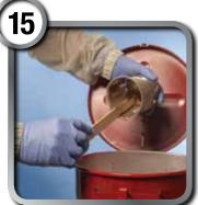
Remove unused material from the liner and place into proper disposal container.
