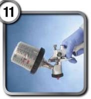
Due to the fact 3M<sup>TM</sup> PPS<sup>TM</sup> is a closed system, painters may now spray their gun completely perpendicular to their intended surface without fear of material dripping on their job.
